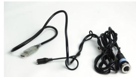
Figure 2. Connection from the PC (USB) to the **YeastForce** (M12 / 8-pin)
