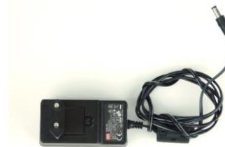
Figure 3. 12 V DC power supply
