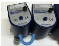
Figure 33: The third cartridge must also be placed at an angle of 10° from left to right. When removing the cartridges, start from left to right.
