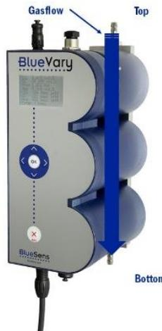
Figure 37: Gas flows in the **BlueVary** "from top to bottom" so that liquids can be flushed out.
