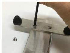
Figure 28: Fastening the mounting plates to the flow adapter
