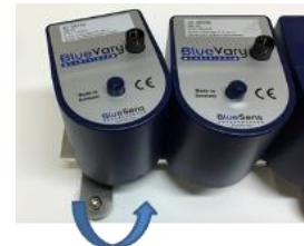
Figure 68: First step in removing the cartridges
