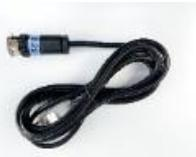
Figure 41: Blue RS232 sticker on the USB adapter of cable D
