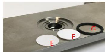
Figure 25: **BlueVary** filter and seal
