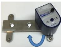
Figure 31: The first cartridge must be placed on the right side of the flow adapter.
