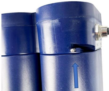
Figure 36: Engaged interlock for the main unit / cartridge
