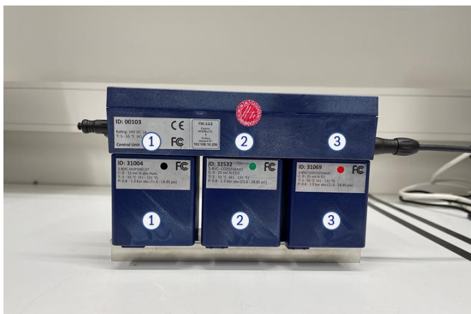
Figure 2: Exemplary illustration of the identification of the slots by stickers on the back of the BlueVary
