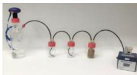
Figure 33: Example installation for a BMP test station with CO<sub>2</sub> absorber and H<sub>2</sub>S absorber
