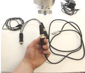
Figure. 18 Connection KA-00015 to KA-00025
