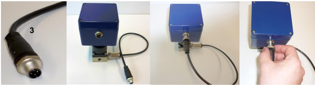
Fig.38: connection pressure sensor to gas sensor and flow adaptor steel (optional accessories)
