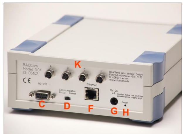
Fig. 32: Connections on the BACCom12
