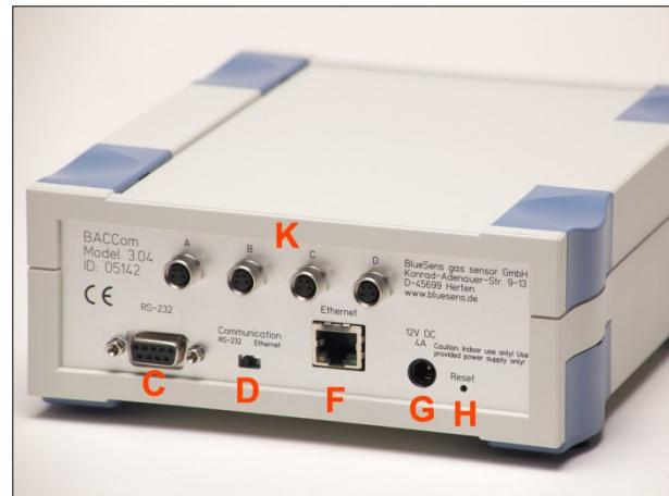
Fig. 25: Connections on the **BACCom12**
