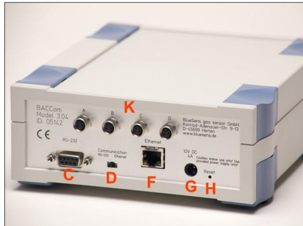
Fig. 38: Connections on the **BACCom12**
