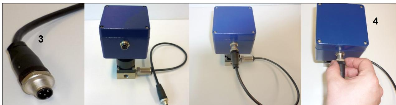
*Fig.46: connection pressure sensor to gas sensor and flow adaptor steel (optional accessories)*
