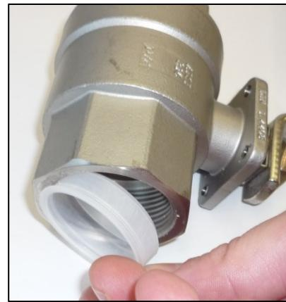
Fig. 15: Removal of the plastic cap
