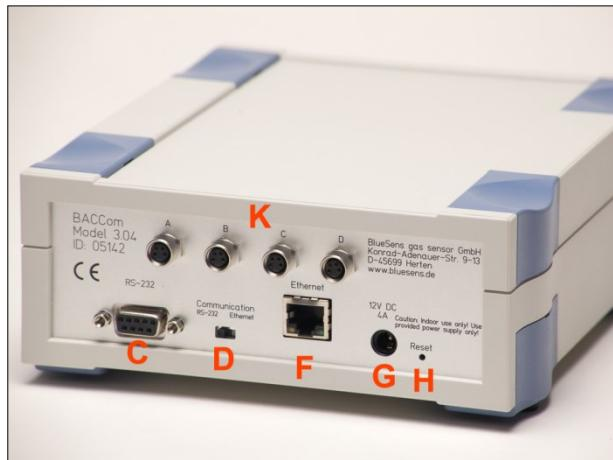
Fig. 30: Connections on the **BACCom12**
