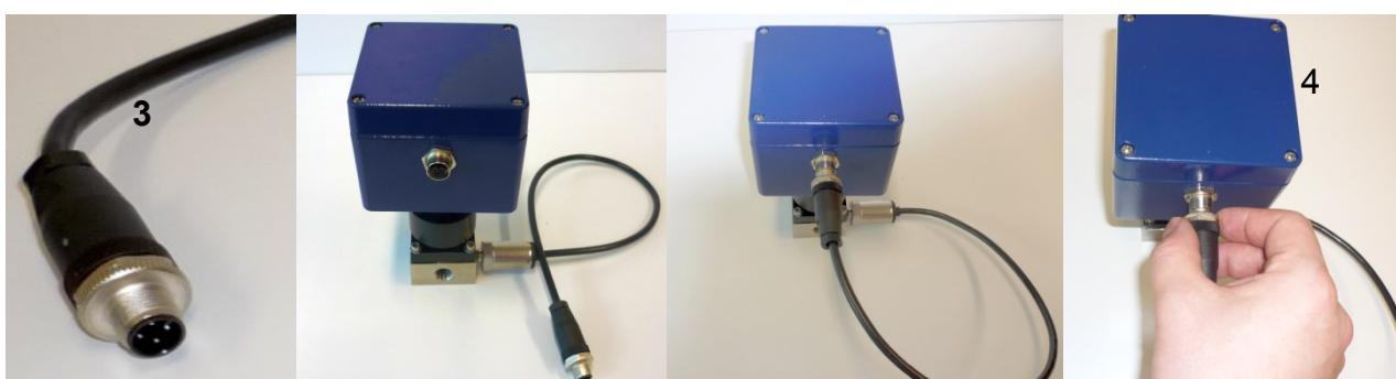
*Fig.37: connection of pressure sensor to gas sensor*
