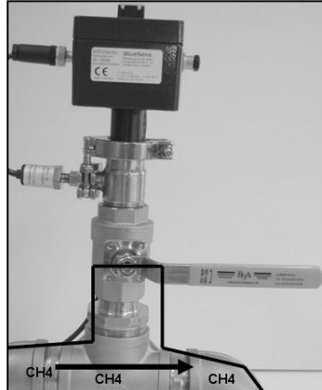
Fig. 19 valve closed
