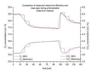
The reaction of the cultures to the event after 2h running time are clearly visible in both gas profiles.
