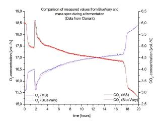
Due to the continuous measurement and the resulting higher data density, the BlueVary shows the events even earlier in some cases, since the reaction of the organism to the addition of the nutrient solution can be detected immediately (2h) and also the time at which the substrate is completely consumed after 18h can be detected more quickly.
