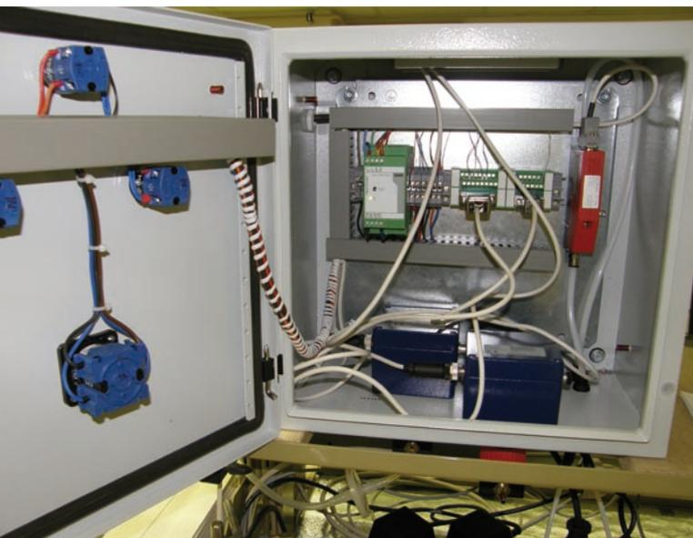
Figure 1: A) self assembled off gas analyser
