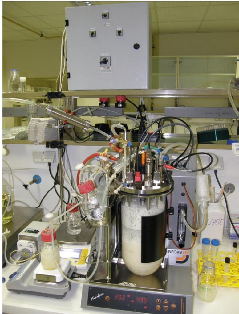
Figure 1: B) bioreactor with off gas analyser
