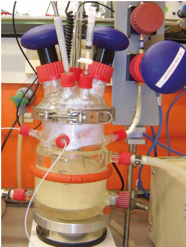
Figure 1: Stirred unit reactor with connected CO<sub>2</sub>, O<sub>2</sub> and ethanol sensors
